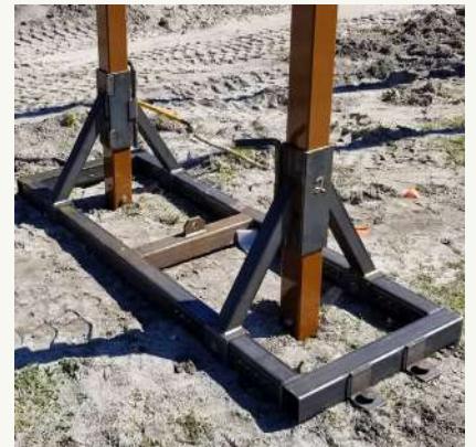
WAGNERS PILING JIG
