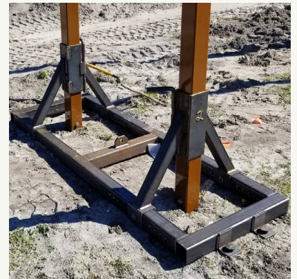
WAGNERS PILING JIG
